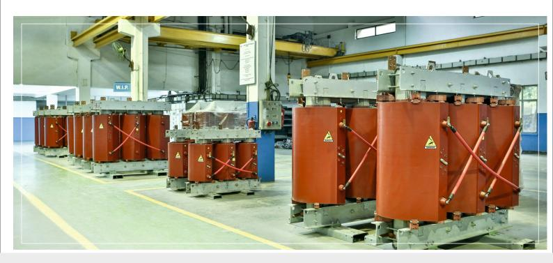
Cast Resin Transformers range up to 5000 KVA (Air Natural/ Air Forced) with a maximum voltage rating of 36 KV/170 KV BIL. It's more than just a technology. It's a concept of safety, reliability and conformity for over 37 year with the principles of environment protection. VPI design transformer manufacturing range is up to 6.5 MVA, 11 & 22 KV class. CRT design transformers ranging from 25 KVA to 5 MVA/11,22 & 36 KV class.
