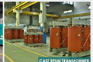
CAST RESIN TRANSFORMER
